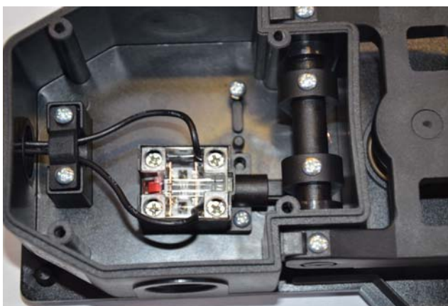
Connect wire to terminal 13 and 14 in foot pedal.
