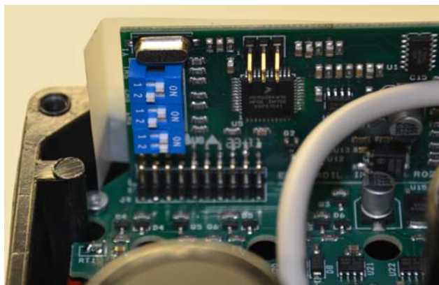
Adjust dip-switch according picture.
