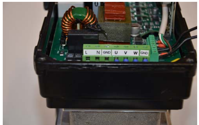
Connect phase to L and zero to N. Ground to GND. Connect foot pedal to terminal 1 and 4.
