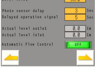
ACTUAL LEVEL OUTLET is the level measured by the sensor (2). This value is used for calculating the feed belt speed, depending on which setting is chosen under FLOW. If the AUTOMATIC FLOW CONTROL is OFF, Evenflow will operate at a constant speed in relation to the setting under FLOW.
