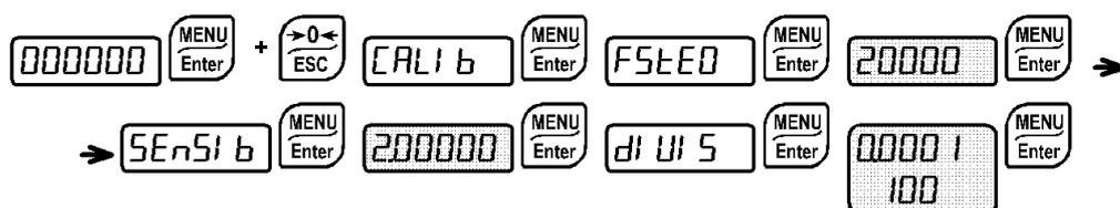
**This function allows the load cell rated values to be set.**
