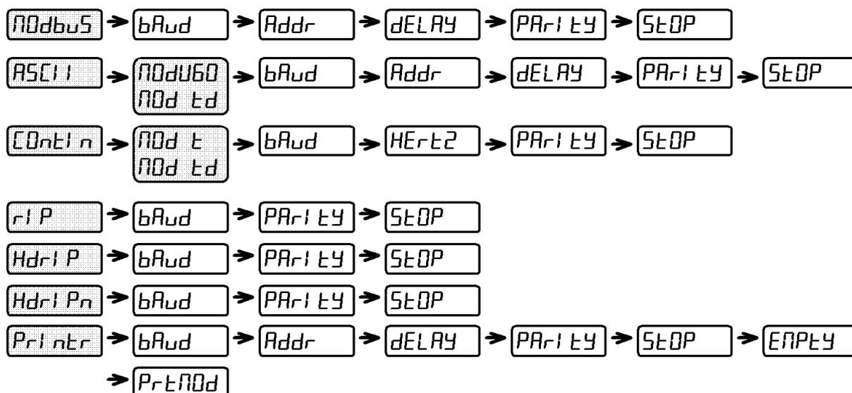
According to the chosen protocol only the necessary settings will be displayed in sequence (see diagram here above).
