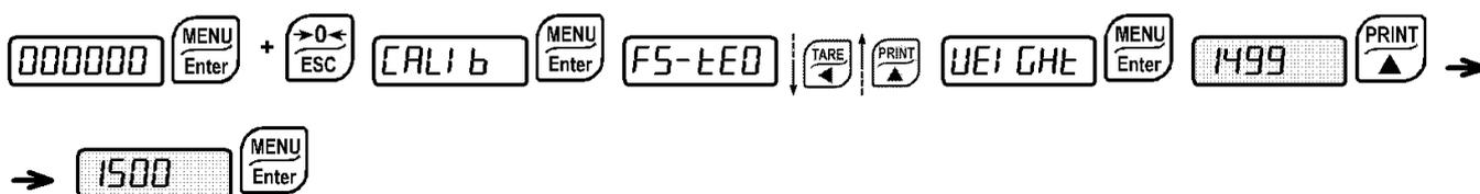
After having performed the **THEORETICAL CALIBRATION** and **TARE WEIGHT ZERO SETTING**, this function allows correct calibration to be done using sample weights of known value and, if necessary, any deviations of the indicated value from the correct value to be corrected.
